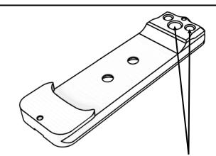
Using the AP-606 without using a quick-release The 3/8 and 1/4 inch holes in the middle section of the plate can be used to attach the foot directly to the threaded stud of a monopod or other lens support equipment, without needing a quick-release clamp.
